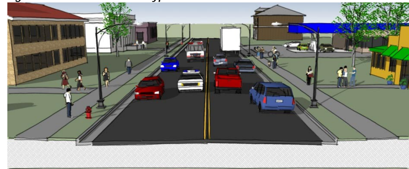
Figure 7.1 Collector Street Typical Section
