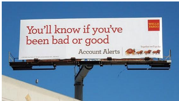
Billboard with a telescoping horizontal member resulting in sign being off center of the vertical support structure.
